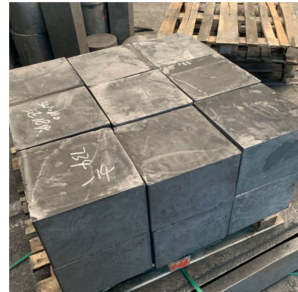
High-purity graphite blocks for ladle refractory linings • ECCN 1C298
