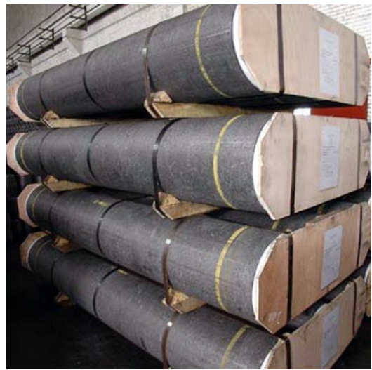
Graphite blocks and logs may be completely exposed or covered with a paper or plastic wrapper to protect the soft surface
