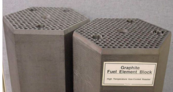
Graphite components of gas-cooled reactors before uranium fuel insertion
