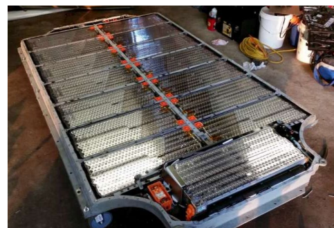
Tesla Model S Battery Pack • 7000 individual lithium-ion cells
