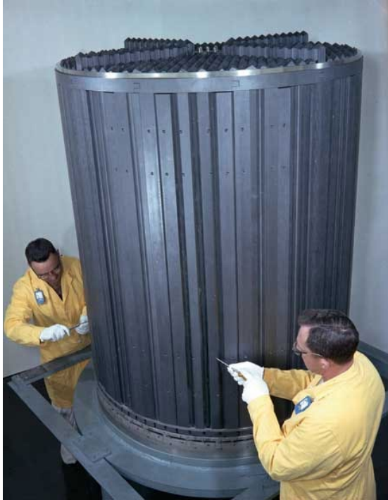
Graphite core from the ORNL Molten-Salt Reactor Experiment
