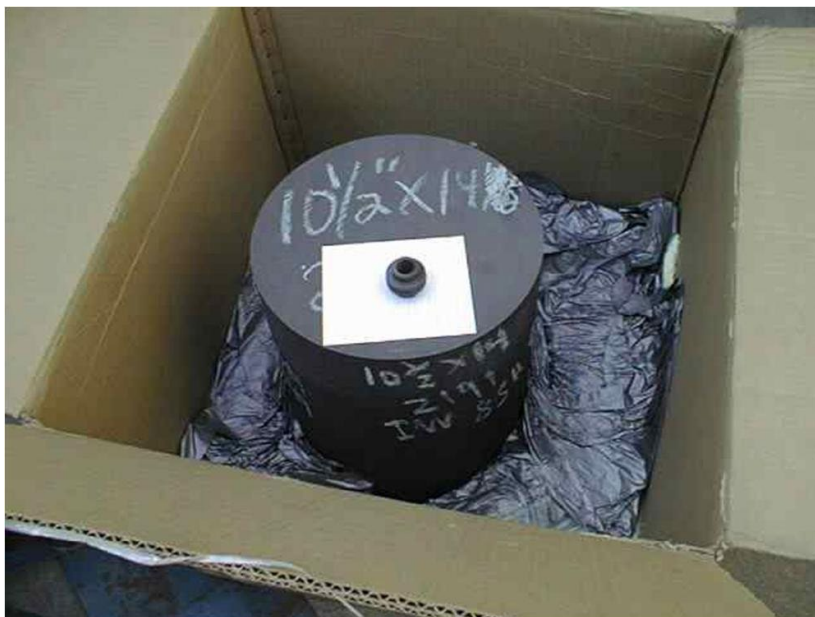
38 mm nozzle sitting on a 10.5" x 14" graphite blank
