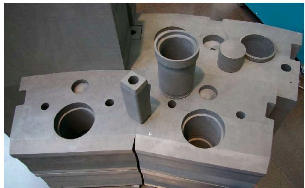
Graphite blocks forming the outer reflector in Pebble-Type HTGR (PBMR)
