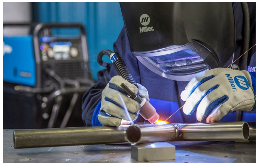
TIG welder using an electric torch as filling material is hand fed into a molten pool.
