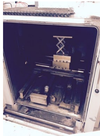
Large vacuum where welding must occur to prevent electron dissipation. ECCN: 2B999.e
