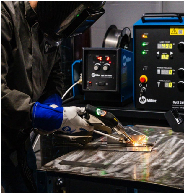
Miller OptX 2 kW hand-held laser welding system. ECCN: 2B999.c
