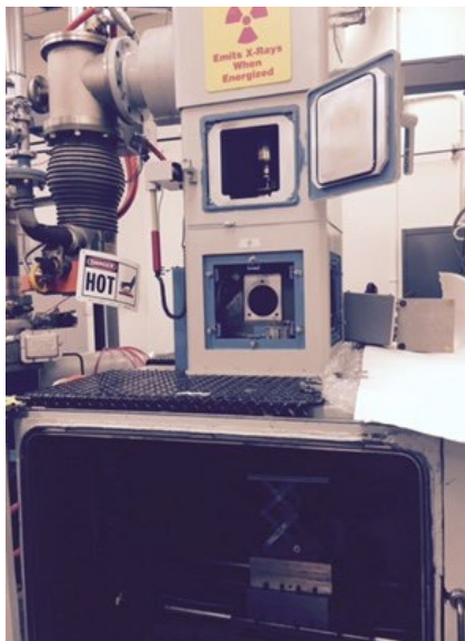
Electron beam welding machine with electron "gun" located outside of vacuum: Note vacuum pump (top left) and trefoil radiation sign (top center). ECCN: 2B999.e
