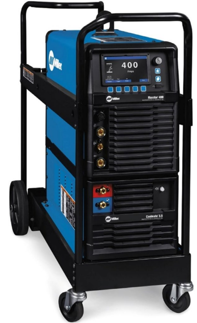
Miller® Maxstar® 400 TIG welder: 208-600 V input, 400 A max output. EAR99
