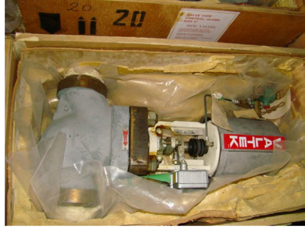
Globe valves EDP for a boiling water reactor.
