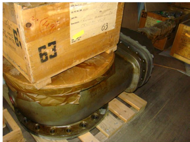
Large gate valve EDP for a boiling water reactor (BWR)
