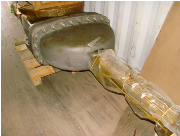
Large gate valve EDP for a boiling water reactor (BWR)
