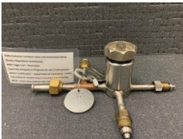
Hoke valve "especially prepared" for UF 6 service. Note flanged piping connections. EDP (10 CFR Part 110).
