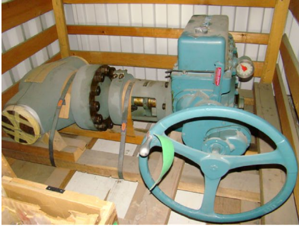
Globe valves EDP for a boiling water reactor.
