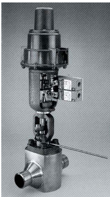
A diaphragm-actuated Monel® bellows seal valve with limit switches for UF6 service. Note the optional detection port with a long tube for monitoring and early detection of bellows leakage.
