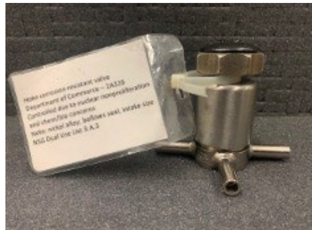
Standard Hoke bellows seal valve (not modified). Dual-use (ECCN 2A226).
