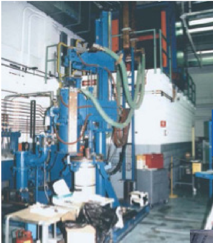
Arc remelt furnace. Heavy, flexible electrical leads and copper busbar visible near center of picture.
