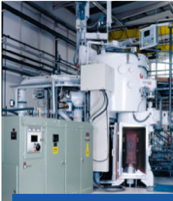
Induction furnace vessel (right) and power supply (left).
