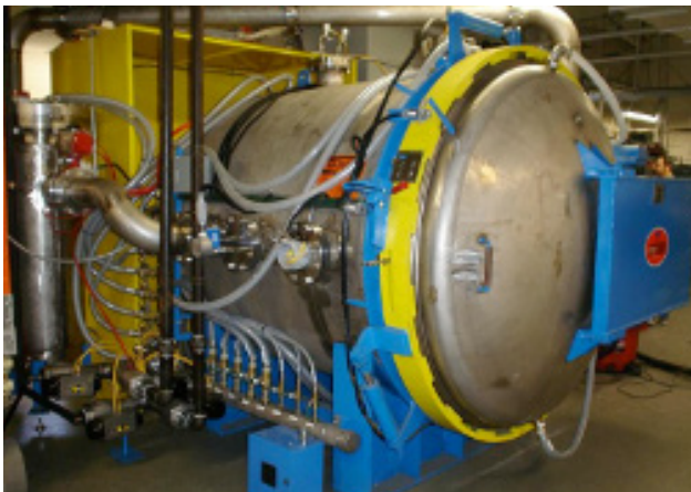
Chemical Vapor Deposition Furnace. A complete system would generally have a chamber, power supply, and programmable control system.
