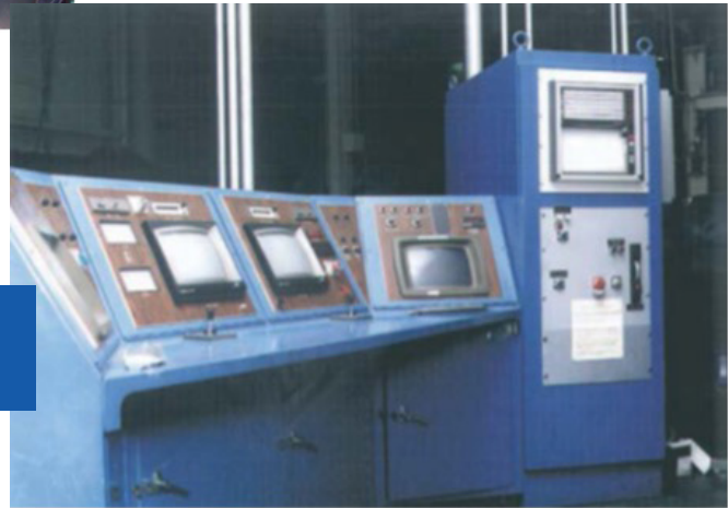
Computer control and monitoring system for an arc remelt furnace.
