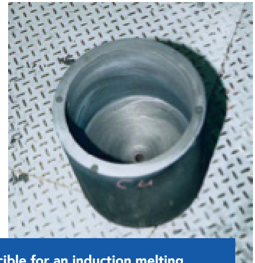
Graphite crucible for an induction melting furnace.
