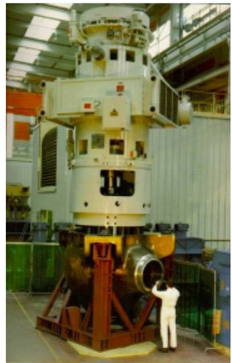
Primary coolant pump EDP for a pressurized water reactor.
