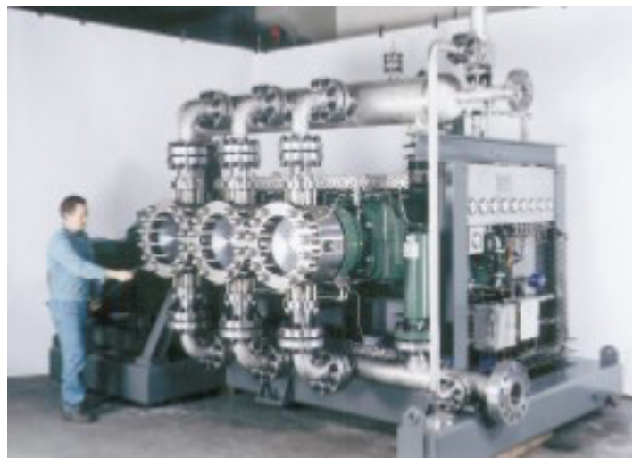
Triple diaphragm pump used in heavy water production
