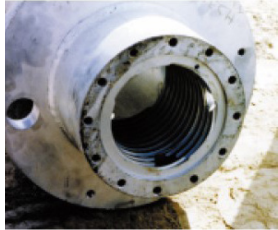
Molecular pump. Note the helical grooves.
