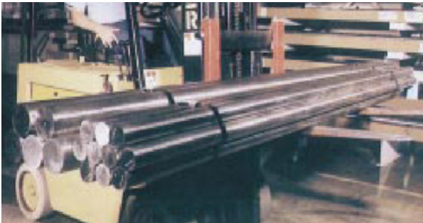
Maraging steel closely resembles stainless steel when newly produced but quickly develops a dark oxide layer
