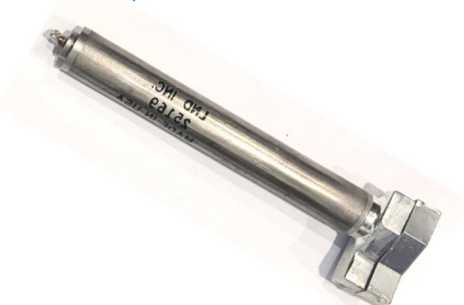
LND Inc. Model 25169 ^3\text{He} neutron detector proportional counter tube. Controlled under ECCN 1C232.
