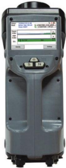
ORTEC "Detective X" ultrahigh resolution HPGe radioisotope identifier
