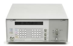
Model 6040 pulse generator from Berkeley Nucleonics Corp. Pulse generators are generally used in scientific experimentation and optics. The Model 6040 has +4 V pulse into 50  $\Omega$  and 700 ps rise time. Note: Model 6040 does not meet the ECCN 3A230 specifications.
