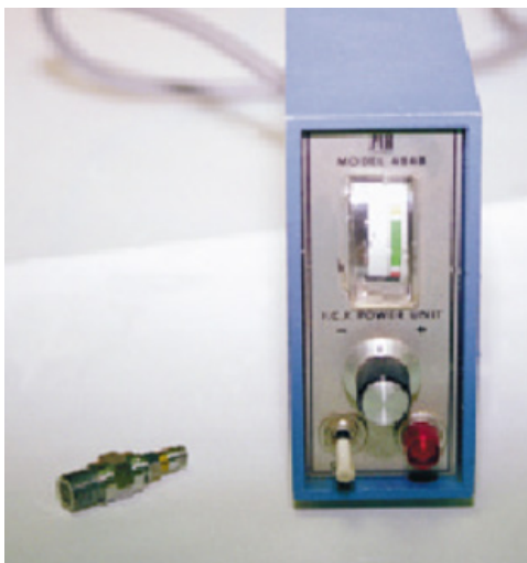
Quartz pressure transducer (lower left) with typical power supply for its operation.
