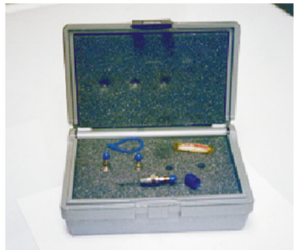
Plastic case with soft foam inserts for shipping quartz pressure transducers. Two transducers are inserted into holes in the foam, and a third transducer lies on top of the foam.
