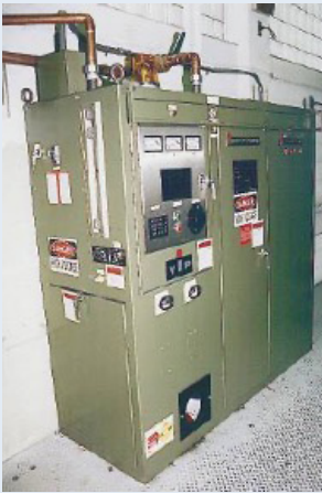
Export-controlled power supply for use with vacuum induction furnace. Note, the multiple high voltage warning signs
