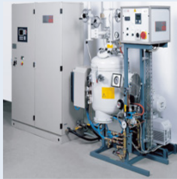
From left to right, power supply, vacuum induction furnace vessel, and controls
