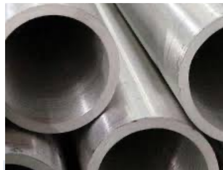
Beryllium-aluminum Grade #140 alloy tubes 60% beryllium and 40% aluminum Controlled by ECCN 1C230 (beryllium >50%)
