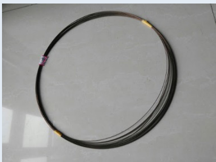
Galfenol wire (FeGa alloy; size 0.8 mm; magnetostrictive material)
