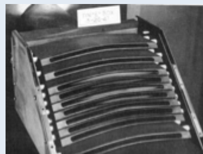
EMIS collector consisting of graphite receivers designed and spaced to collect the 10 stable isotopes of tin
