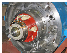
Radial magnetic bearing for positioning a rotor using four electromagnets
