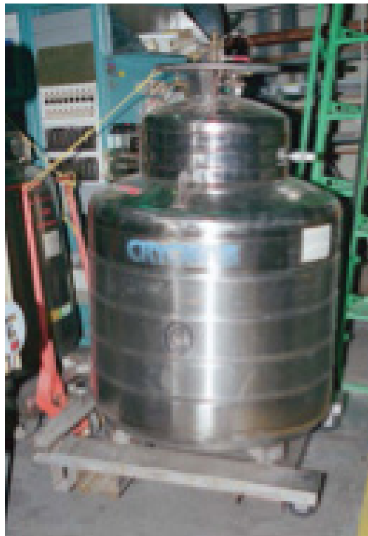
Example of a Dewar for storing liquefied gases required for superconducting electromagnet operation
