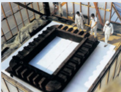
EMIS magnet coils especially designed or prepared for an alpha calutron for uranium enrichment
