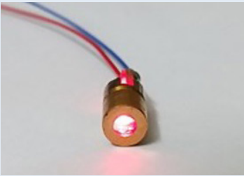
A simple and low power metal enclosed laser diode. Not controlled.
