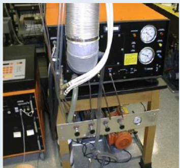
Excimer laser with gas connections and pressure gauges. ECCN 6A005.d.4.
