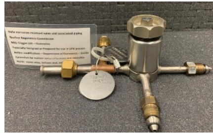
Hoke valve "especially prepared" for UF_6 service.
