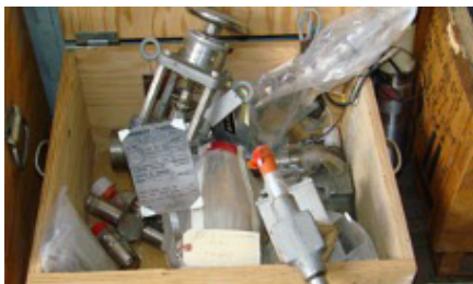
Crate of EDP valves for reactor service with attached N stamp nameplates.
