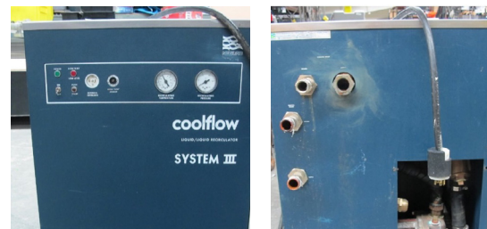
NESLAB System III heat exchanger. Dimensions: 34 in. H x 23 in. W x 27 in. D. Weight: 206 lb. Note the four piping connections and markings.
