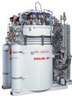
Helium refrigeration unit. Performance ranges: Heat removal capacity is 100 W to 1 kW at 4.5 K. Electrical consumption is 50–250 kW.
