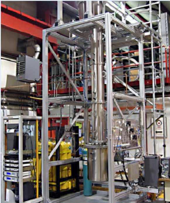
Cryogenic distillation column at Fermi National Accelerator Laboratory.
