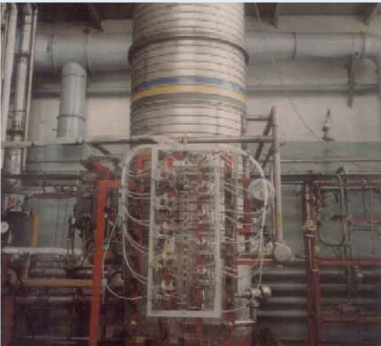
Hydrogen Isotope Separation Test Assembly in Russia. The cryogenic distillation column shown is 18 ft (5.5 m) in length with an internal diameter of 12 in. (30 cm), and an outer 48 in. (120 cm) diameter vacuum jacket.
