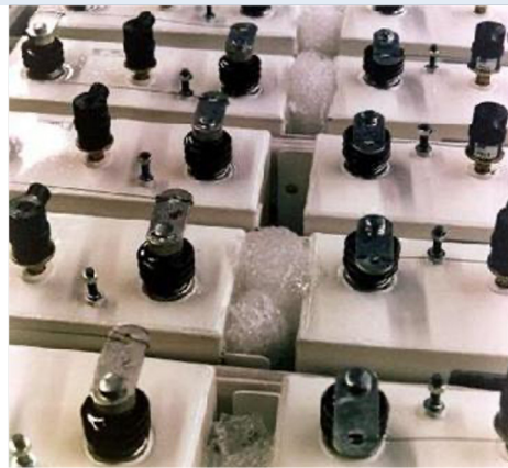
Filter capacitors packed for shipping. Note the wires shorting the terminals.
