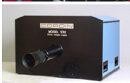
Charge coupled device-based RM streak/ framing cameras do not have the distinctive circular shape
