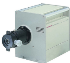
Modern electronic streak camera by Hamamatsu Photonic Division, Japan (Model C5860)
