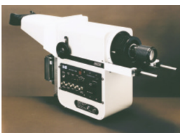
Electronic camera capable of both streak and framing operation (measures 37 in. long and weighs 59 lb).
